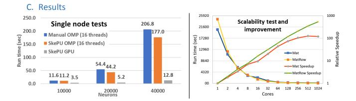
Single node tests were conducted on a 2x Intel Xeon Gold 6138, 2x20 H/T cores with 128 GB RAM that integrates an nVidia Tesla V100 GPU with 32GB VRAM. We noticed that applying the EXA2PRO framework, and more specifically SkePU, results in efficient use of parallel hardware, including GPU.
